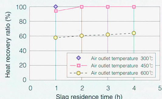
Fig. 5 Heat recovery from coagulated slag chip
